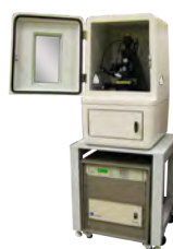
TI 750H Ubi™ (Testing up to 10N)
