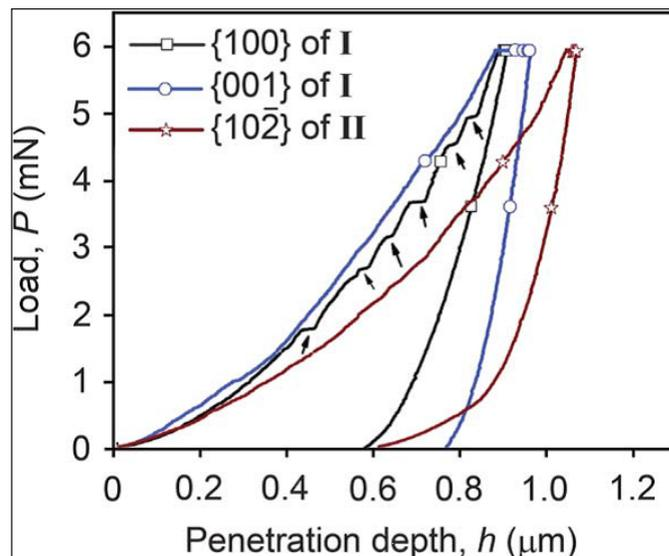
Figure 2: Representative load versus depth curves for all three faces examined, with popins indicated by arrows for the loading curve of {100} of I. [Chem. Sci., 2011, 2, 2236–2242] – Reproduced by permission of The Royal Society of Chemistry.
